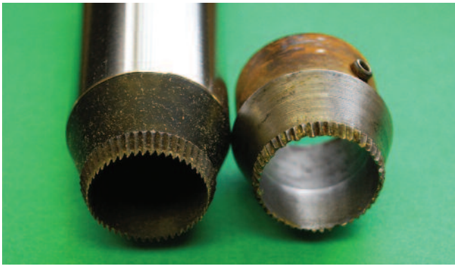
Figure 2. Compare the sharp (left) and dull (right) 3/4-inch diameter serrated tip on a 1-inch tube of a Penn State drill-type single-sample probe. If your probe tip is dull, sharpen it or get a new tip. For these serrated tips, it's easiest to buy a replacement tip when yours is dull.
