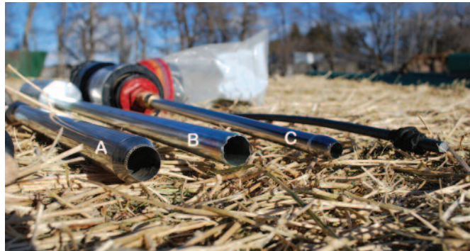
Figure 3. Compare (A) the 3/4-inch diameter serrated tip on a 1-inch tube of a Penn State drill-type single sample probe, with (B) the 3/4-inch diameter scalloped tip on a tube of an AMS drill-type multi-sample probe, and (C) the 1/2-inch diameter scalloped tip on a Star Quality multi-sample push probe. Probes B and C come with a sample container. The remaining item is a wooden or plastic plunger (dowel) that comes with probes to help remove core samples from the probe.
