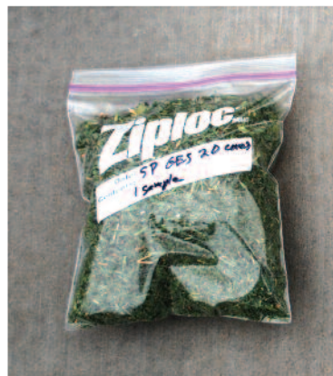
Figure 4. This 1/2-gallon sealable freezer bag holds samples of 20 hay bale cores weighing a total 135 grams or 0.3 pound. They came from a 1/2-inch diameter probe. The bag is labeled to enable lot-identification after lab results are in.
