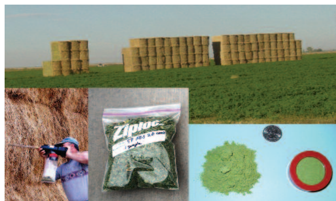
Figure 1. The amount of ground forage sample analyzed by chemistry or near infrared reflectance spectroscopy (lower right) is small in relation to the core sample (lower left and center) of one lot of hay that is sent to a lab. The stack of hay in the background is 3 separate lots from the same field, each from a different cutting.
