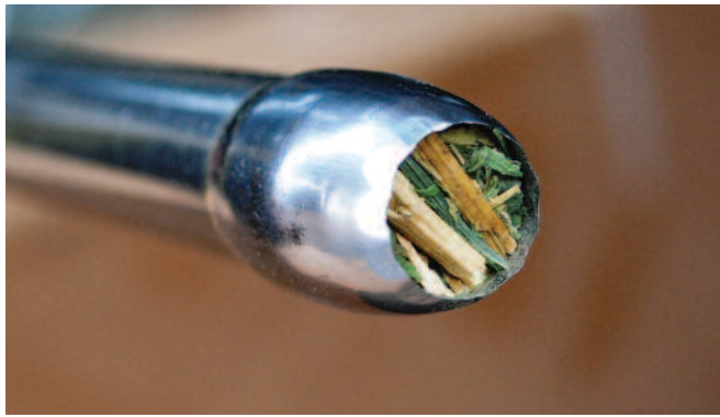
Figure 5. A sharp core tip inserted correctly will cut stems and retain leaves in the same proportion as in the bale. This 0.5-inch tip is on the Star multi-forage sampler and is scalloped and expanded, which allows easy insertion by pushing and easy extraction.
