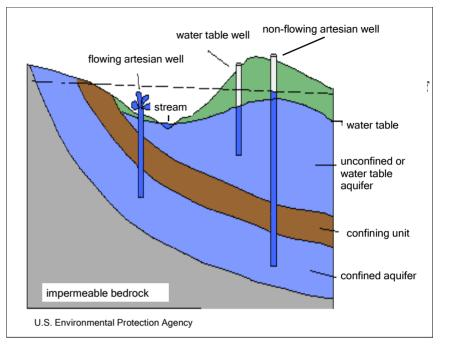
Confined aquifers are sometimes described as *artesian aquifers*. Artesian is anywhere pressure head brings the water level above the top of the aquifer. A well is flowing artesian where the pressure head brings the water level above ground surface.
