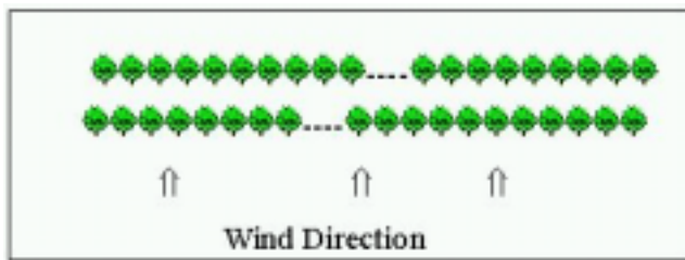
Figure 2. Angling the gap on a shelterbelt can prevent wind tunneling through gateways etc.
